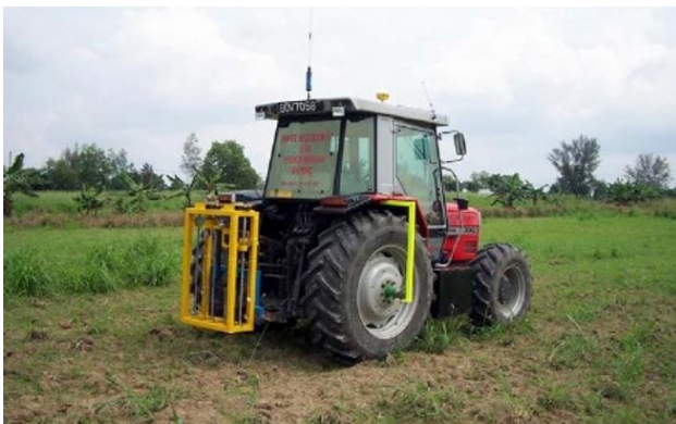
Fig. 5. The instrumented tractor with mounted soil penetrometer – shearometer unit
