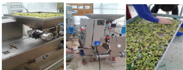
Fig. 2. Oil mill. The process of olive washing and cleaning
